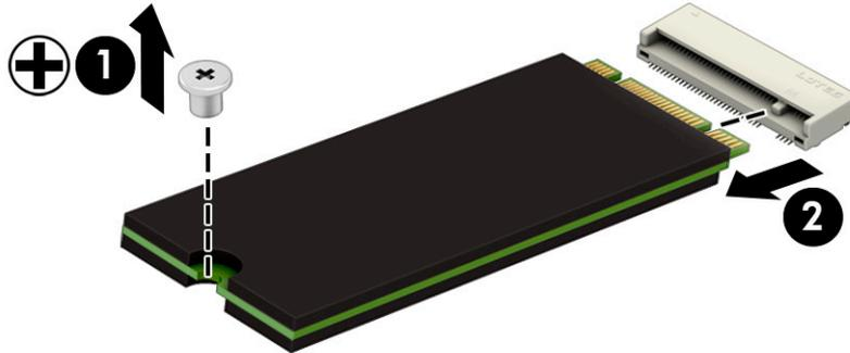
To install the solid-state drive module, reverse the removal procedure.
