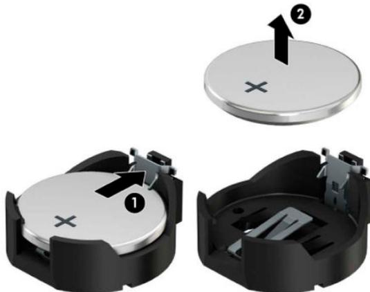
3. Slide the replacement battery into position, positive side up. The battery holder automatically secures the battery in the proper position.
