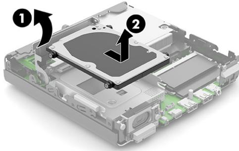
2. Lift the connector latch on the system board, and then pull the tab **(1)** to disconnect the hard drive cable **(2)**.
