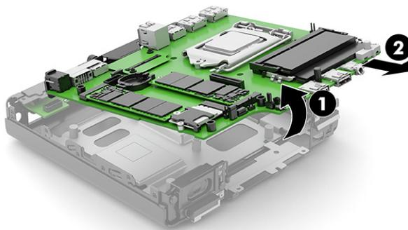
To install the system board, reverse the removal procedures.
