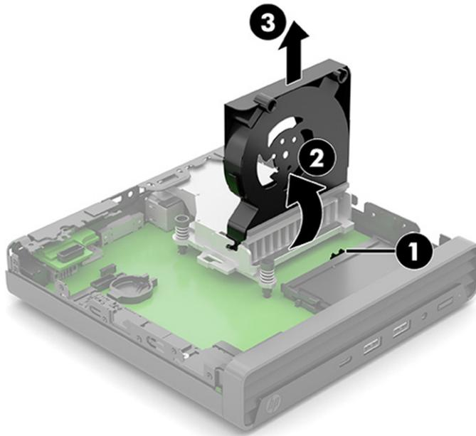
To install the fan, reverse the removal procedure.
