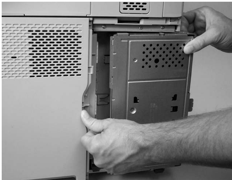
Figure 5-32 Remove the formatter cover and formatter (3 of 3)
