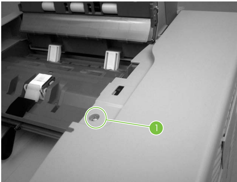
Figure 5-190 Remove the ADF rear cover (1 of 2)
