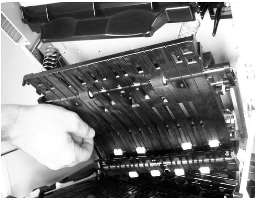
Figure 5-50 Remove the reversing-separation-guide assembly (2 of 2)
