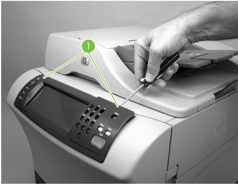
Figure 5-1 Remove the control-panel overlays
