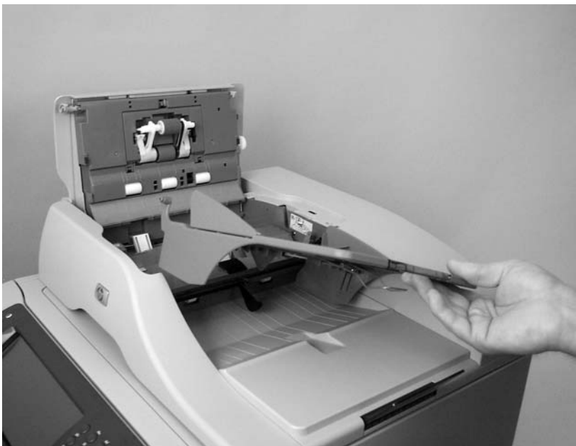
Figure 5-7 Remove the ADF input tray (3 of 3)
