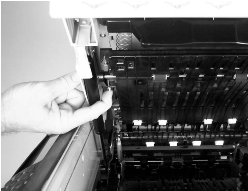
Figure 5-49 Remove the reversing-separation-guide assembly (1 of 2)
