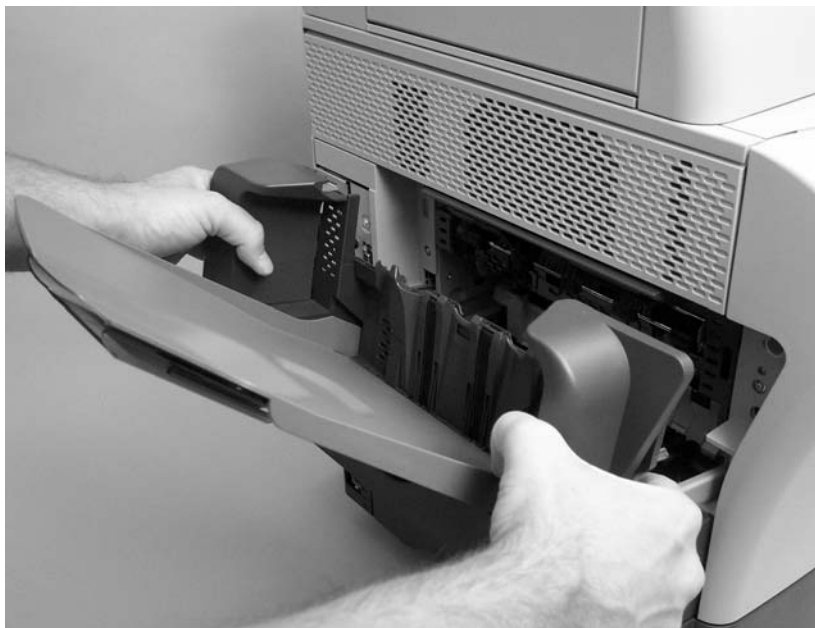
Figure 5-17 Remove the output-bin assembly (2 of 2)
