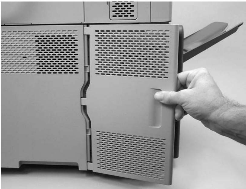
Figure 5-30 Remove the formatter cover and formatter (1 of 3)
