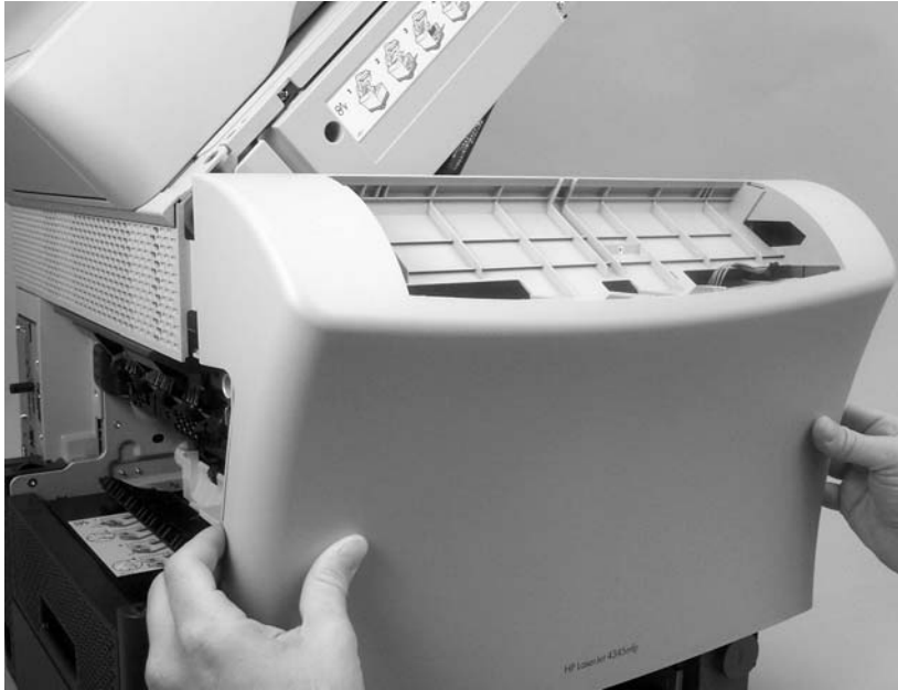
Figure 5-45 Remove the front cover (7 of 7)
