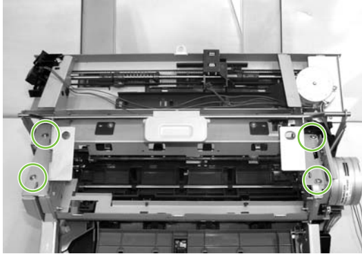
Figure 5-215 Remove the jogger unit (6 of 7)
