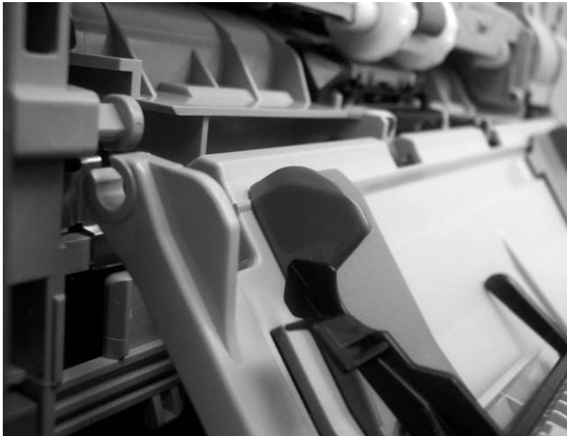
Figure 5-78 Remove the tray 1 assembly (4 of 5)
