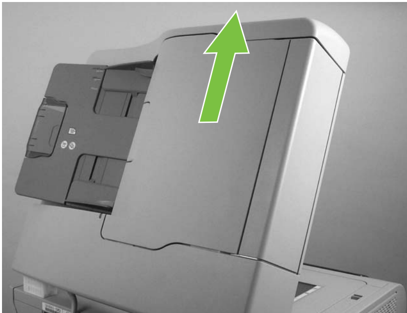
Figure 5-170 Remove the ADF assembly (3 of 3)
