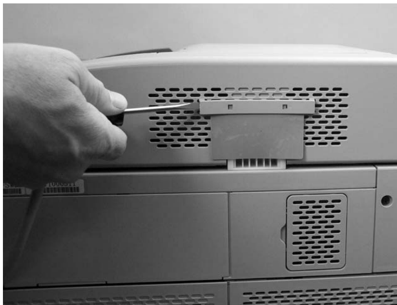
Figure 5-28 Remove the ADF-hinge flap (2 of 3)
