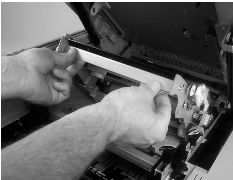
Figure 5-58 Remove the reversing assembly (8 of 8)
