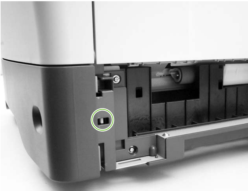
Figure 4-76 Tray 2 jam-access-cover switch, SW105
