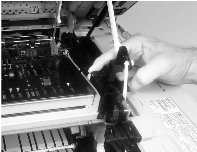
Figure 5-52 Remove the reversing assembly (2 of 8)
