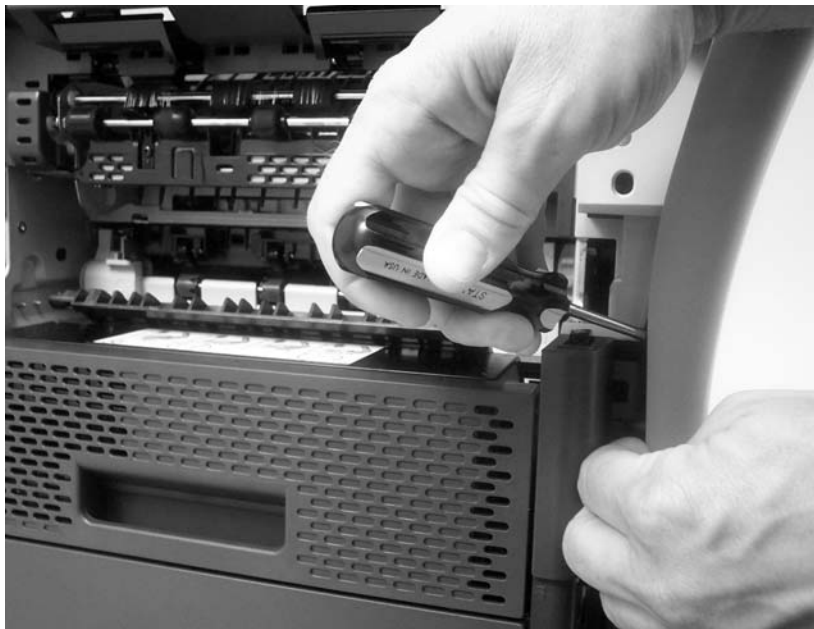
Figure 5-42 Remove the front cover (4 of 7)
