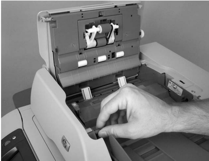
Figure 5-6 Remove the ADF input tray (2 of 3)
