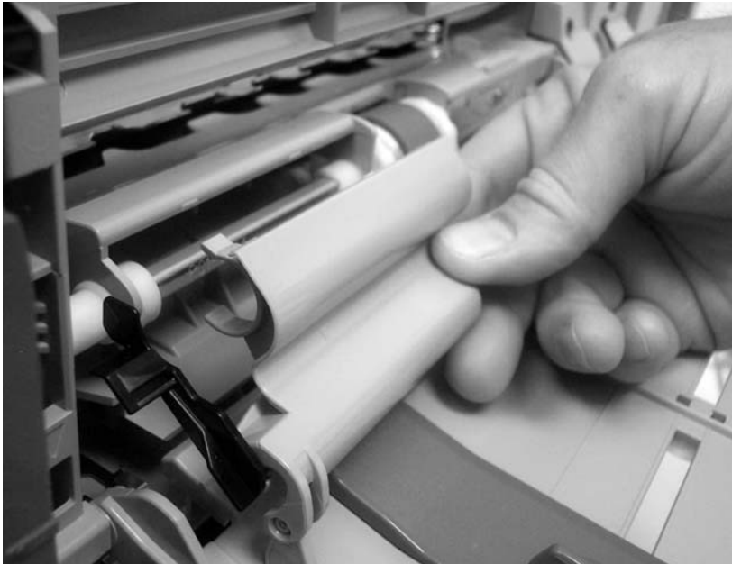
Figure 5-77 Remove the tray 1 assembly (3 of 5)
